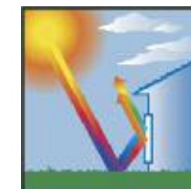
Low-E glass filters long-wave radiation from the sun. This reduces heat gain in the summer, keeping your home cooler.
